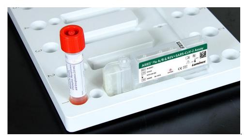
8. Open the cassette cap and place the specimen in the cassette sample chamber by inserting the pipette tip near the bottom of the chamber before expelling the specimen.
